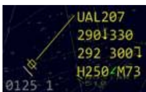
Figure 9–9. Sector Position Accepts Proposed GIM-S Speed
