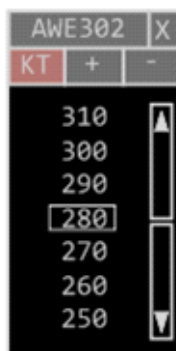
Figure 4–41. Speed Menu Displaying Controller-Entered Speed in Knots
