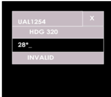
Figure 4–39. Heading Input Error Area
