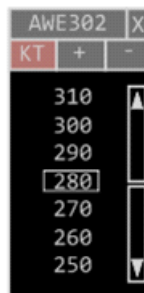
Figure 4–40. Speed Menu Displaying Controller-Entered Speed in Knots
