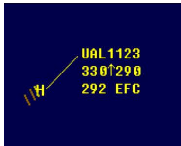
Figure 4-10. Data Block Hold EFC
