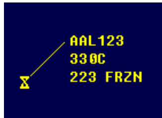
Figure 4–8. Data Block with Frozen Indicator
