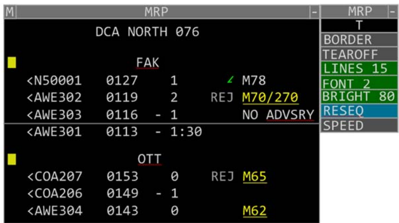
Figure 13–9. Meter Reference Point List View (View Menu)
