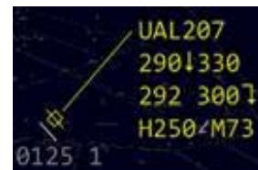
Figure 9–9. Sector Position Accepts Proposed GIM-S Speed
