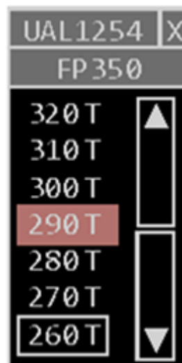
Figure 4–24. Altitude Menu with Assigned Interim Altitude & Flight Plan
