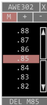
Figure 4–42. Controller-Entered Speed Value in Mach
