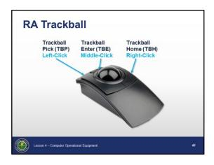
The trackball is used to initiate actions by selecting items from displays and menus using three buttons.
