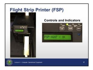
The Flight Strip Printer (FSP) is a thermal printer that uses a fanfold paper supply and cuts the paper after each strip is printed. The front of the printer contains a strip receptacle tray, called a hopper, to receive printed strips.
