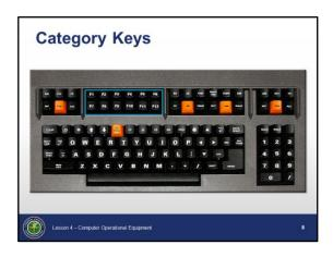
There are 12 Category Keys (F1 through F12) - Any of these keys can be facility adapted to perform other functions such as inserting characters and or spaces to complete a command.
