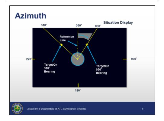
AZIMUTH - The direction of an object from the antenna based on a 360° circle measured clockwise from a reference line.
