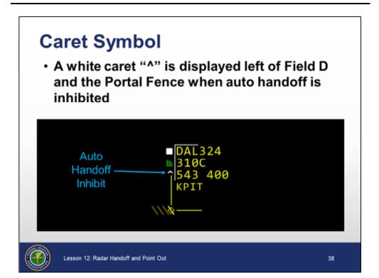
A white caret "^" is displayed to the left of Field D and the Portal Fence when auto handoff is inhibited
