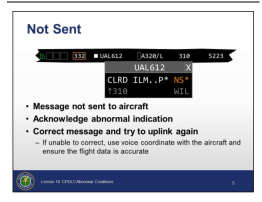
When the system is not able to build the uplink message, the system will automatically close the uplink and set the status to not sent, indicated by NS
